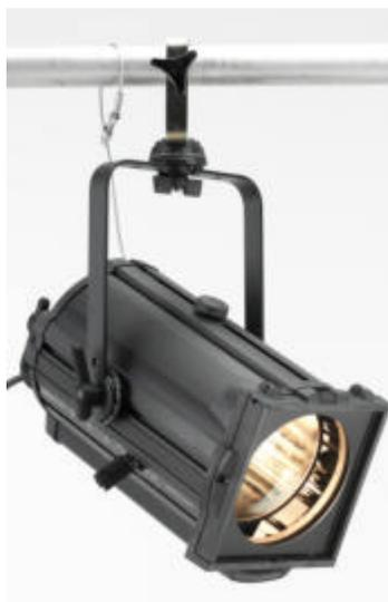
**The Rama High Performance 175 FFT PC (1.0kW / 1.2kW, 175mm lens) provides an adjustable cone of light has a soft edge and is easily blended with adjacent beams to provide even illumination. The custom designed PC lens produces outstanding light output and unmatched beam quality, similar to a profile beam with 114 Hamburg Frost.**
